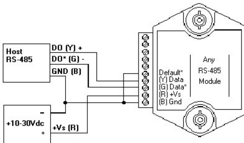
The polarity of the DGH RS-485 lines is indicated above. It should be noted that '(Y) Data' is the Positive (+) line. The '(G) Data\*' line is the Minus (-) line.
