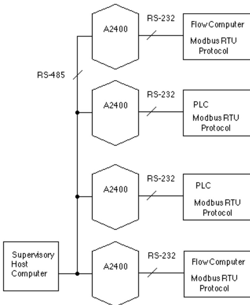
Figure 10.2 A2400 networking several RS-232 devices to a host computer.
