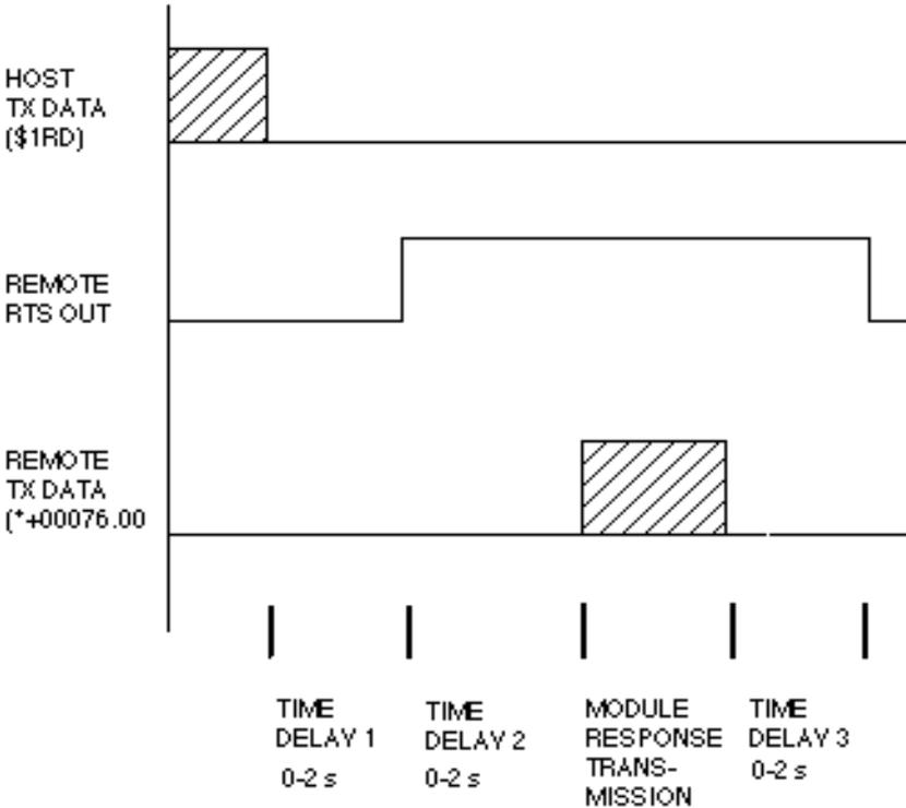
Figure 6.1 Programmable delay times.
