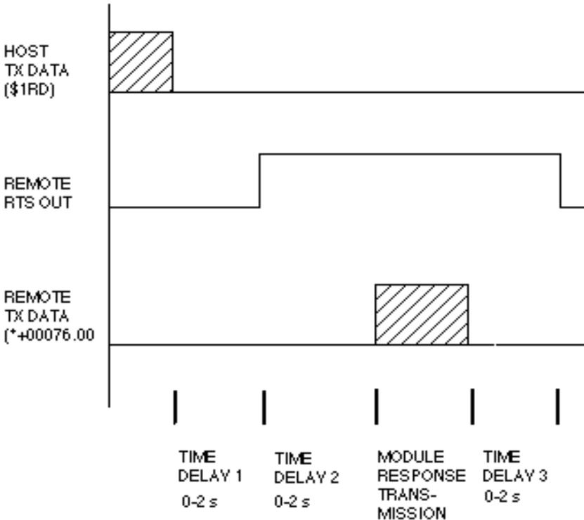
Figure 2.2 Programmable Delay Times.
