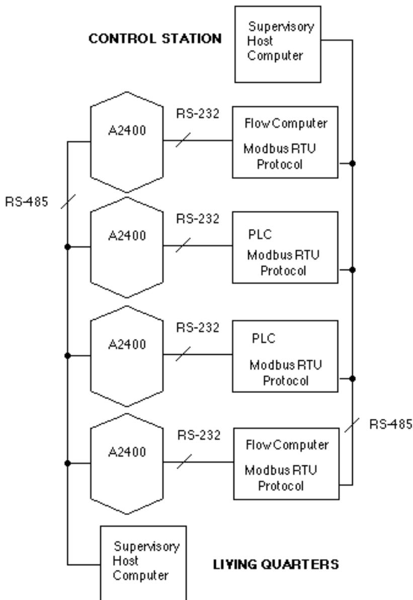
Figure 10.5 Adding secondary control using A2400 modules.
