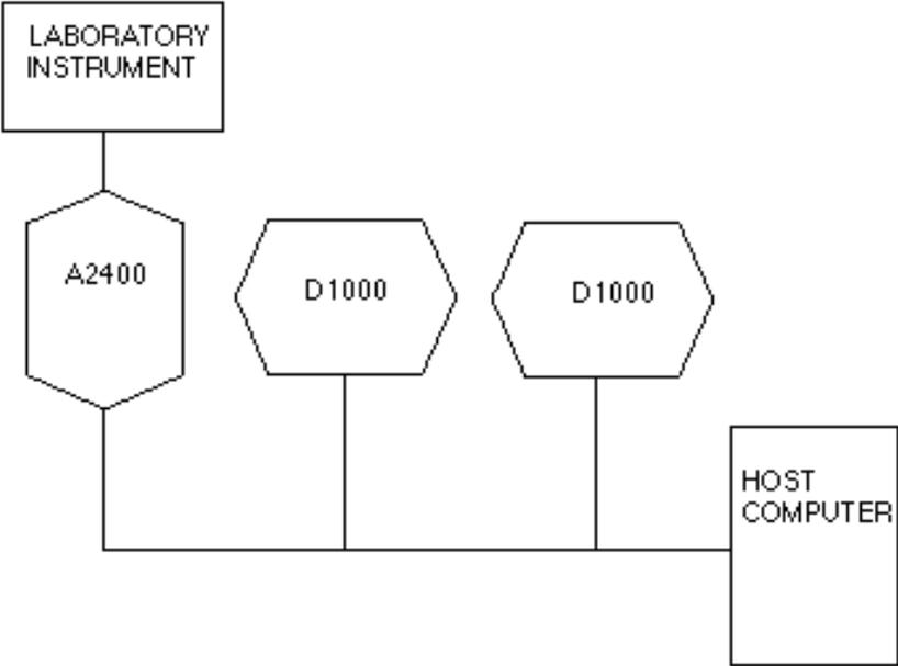
Figure 10.3 A2400 interfacing a laboratory instrument with modules.
