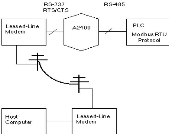
Figure 10.1 A2400 interfacing a PLC to a leased-line modem.
