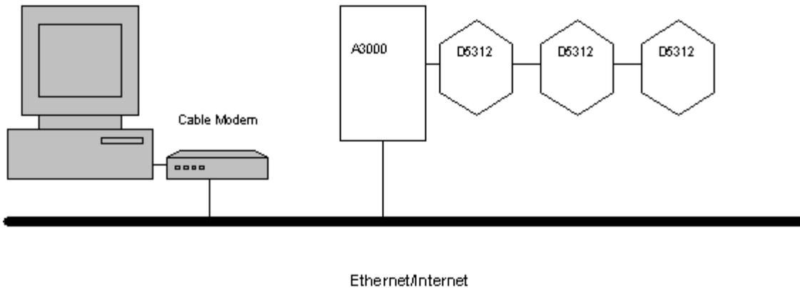
Figure 5.0 RS-485 application using DGH D5000 4-Channel Modules
