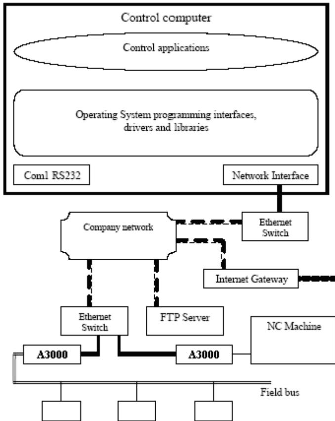
Figure 2.0 Network communication structure.
