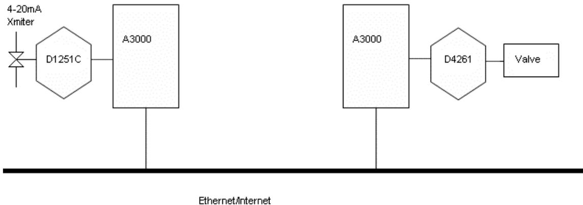
Figure 10.0 Continuous Analog Input/Analog Output Using Serial Tunneling
