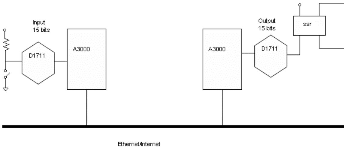
Figure 11.0 Continuous Digital Input/Digital Output Using Serial Tunneling
