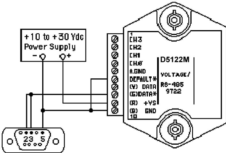
**Note:** If using a DB-25 connector ground is tied to pin 7.
